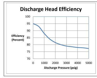
NOTE: With an increase in discharge pressure, the volumetric pumping efficiency of the pump head decreases as shown in the chart.
